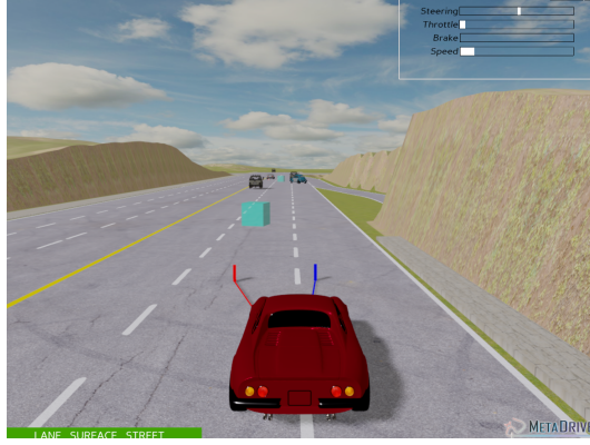
Figure 2: Policy visualization in image space. The predicted rollout of the learned policy is shown as a blue curve, while the expert policy rollout is shown as a red curve, overlaid on the ego-view.
